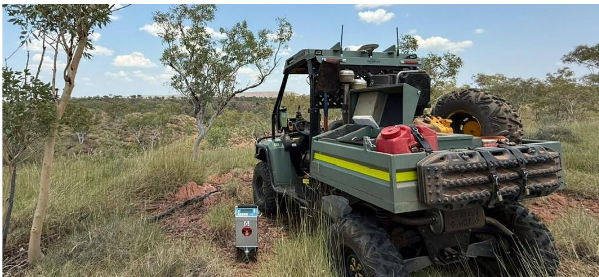
Photo 1: Blue Devil project gravity station data reading station in action.
