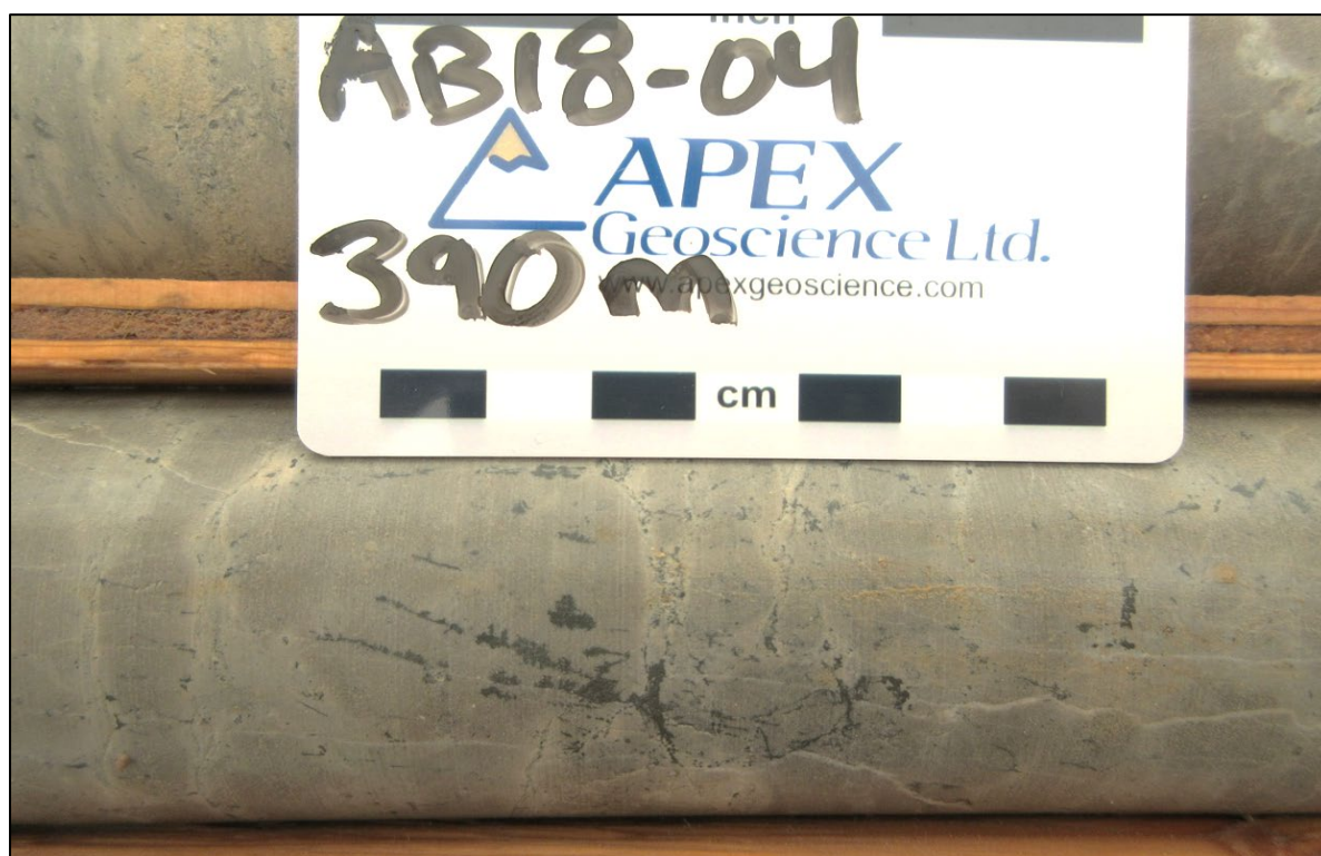
Figure 1: Visual sulphide (dark grey mineral, interpreted to be chalcocite) at 390m downhole in drill hole AB18-04. Chalcocite is a copper sulphide mineral that contains approx. 80% Cu. This drill hole has not yet been sampled, and visual estimates of sulphide type, quantity and habit should not be considered a substitute for laboratory assays. Laboratory assays are required to determine the widths and grade of mineralisation. Portable XRF has been used to assist logging.
