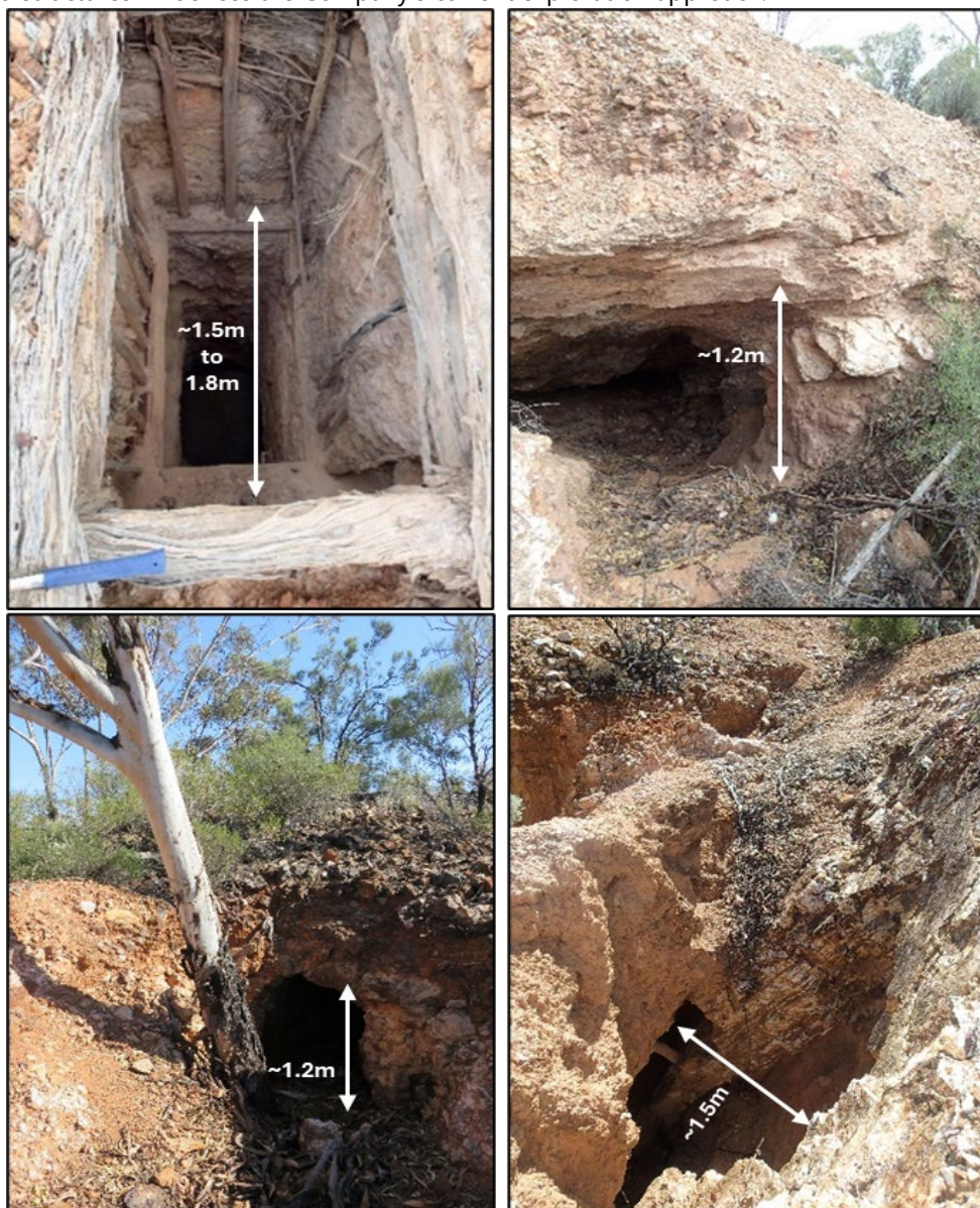
Figure 13: Examples of the range of styles and varying complexity of 1920s historical workings along the Foster Gold Belt. Workings shown above at the following prospects: Jubilation prospect (top left and right); Hustler (bottom left); Cooe (bottom right).
