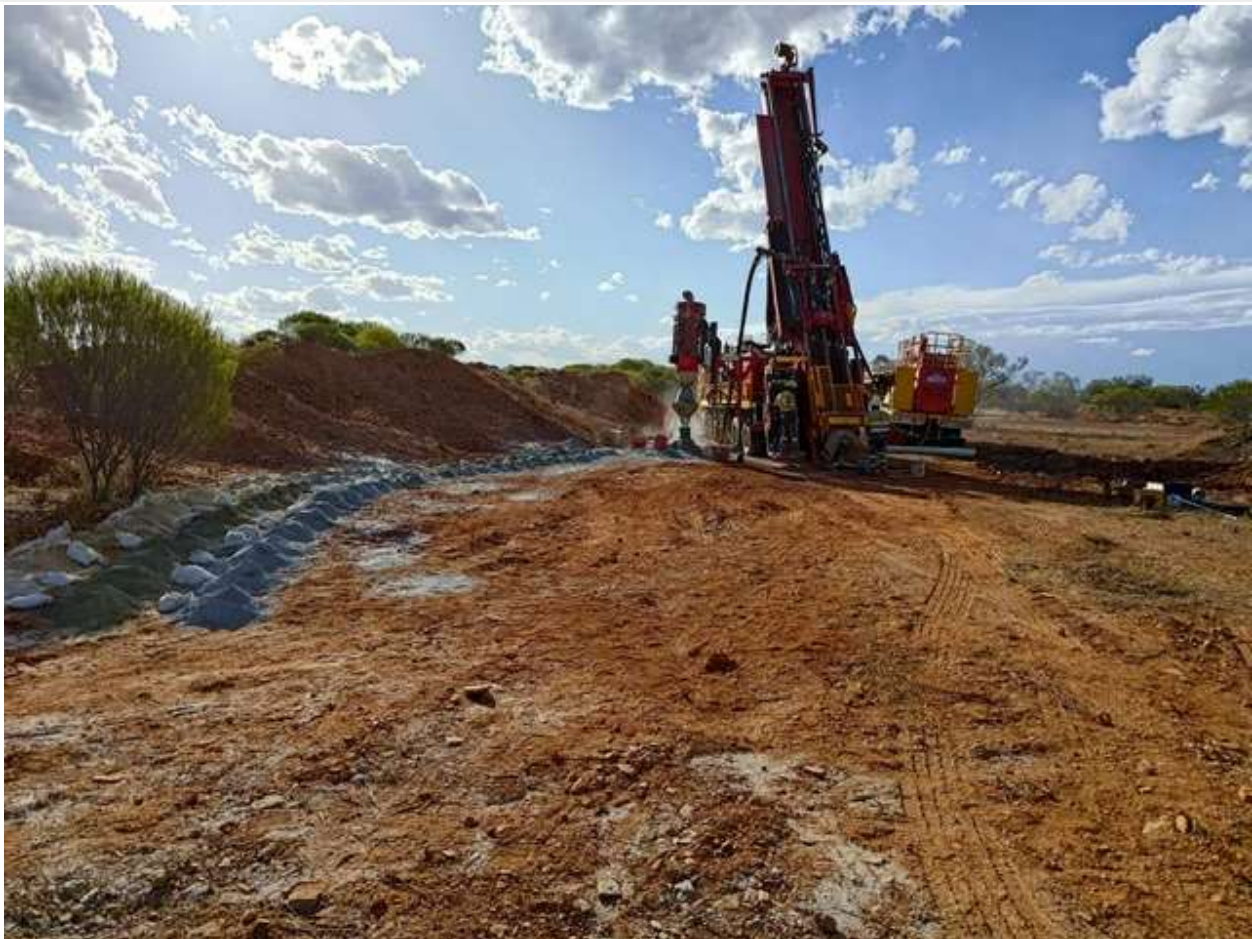
Figure 1: RC Drilling in progress
