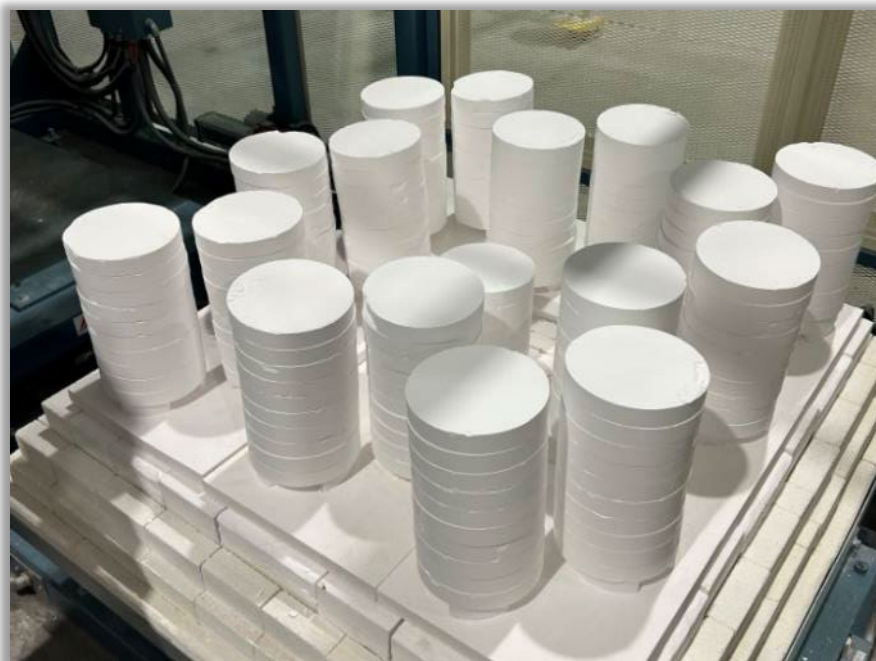
A production batch of densified, sintered HPA disc tablets (Approx value of product shown = US$4K, each tablet ~850g with density of >3.5g/cm 3 )
