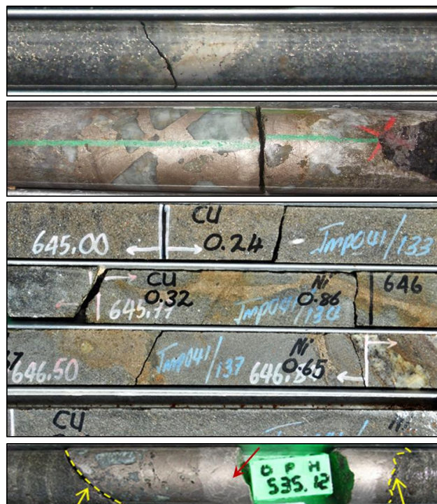
Figure 3: Type 2 mineralisation hosted by all lithological units at Jacomynspan. Including massive sulphide stringers, with higher tenor (>4% Ni), and which has coarse loop texture (red arrow) (JMP038) (refer ASX release 8 March 2018).
