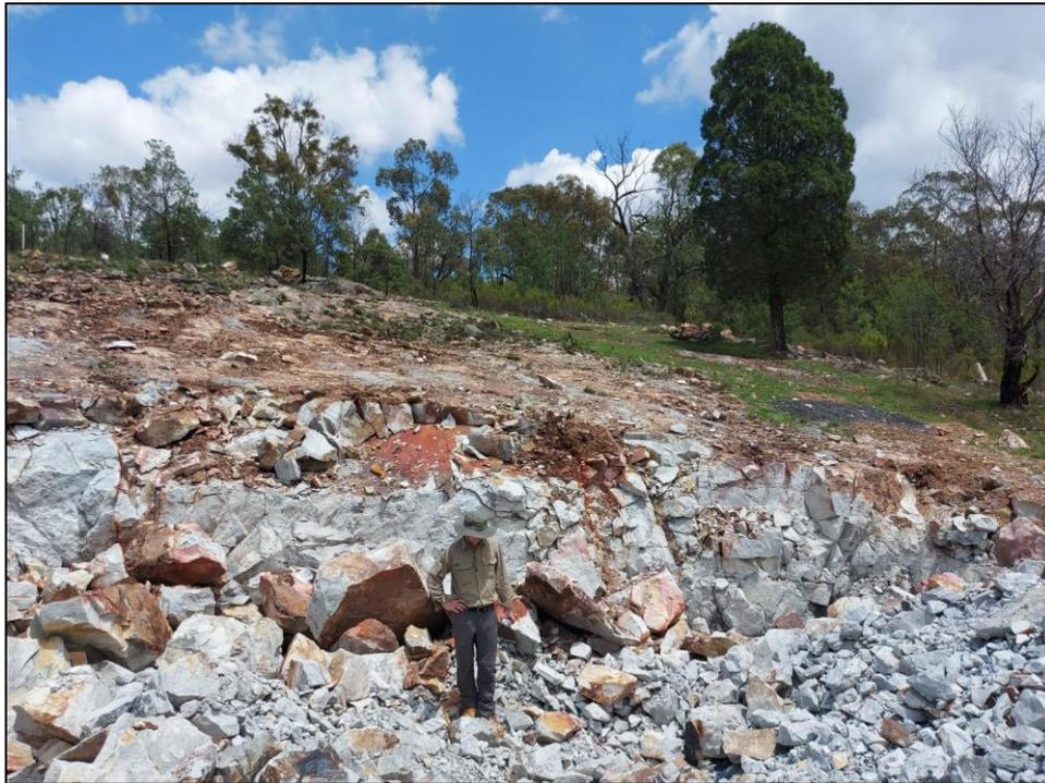
Figure 2: Bulk sample blast site showing mineralised fractures.
