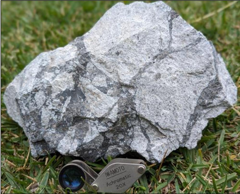
Figure 3: Material from bulk sample site with grey fracture/breccia fill minerals of silver sulphides such as acanthite ( $Ag_2S$ ), galena ( $PbS$ ), sphalerite ( $ZnS$ ).
