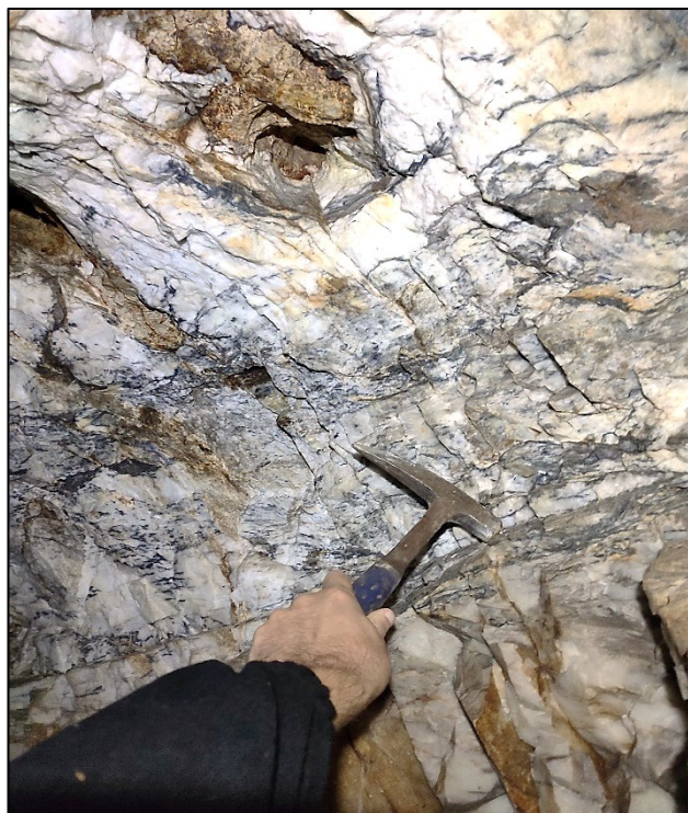
Figure: Kovacevac, flat-laying barite vein ~1m wide with sooty mineralisation (tetrahedrite-sphalerite-galena)
