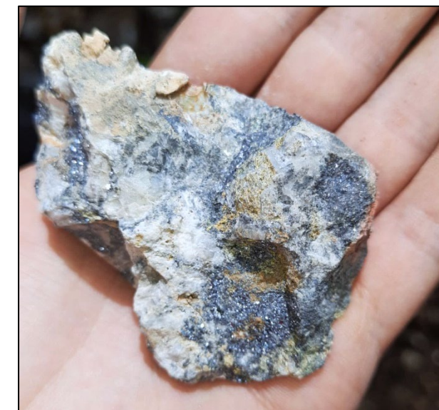
Figure: Bag, tetrahedrite-sphalerite-galena mineralisation
