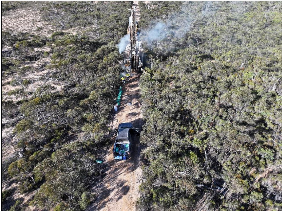
Figure 1: Aircore drilling at the Salazar project
