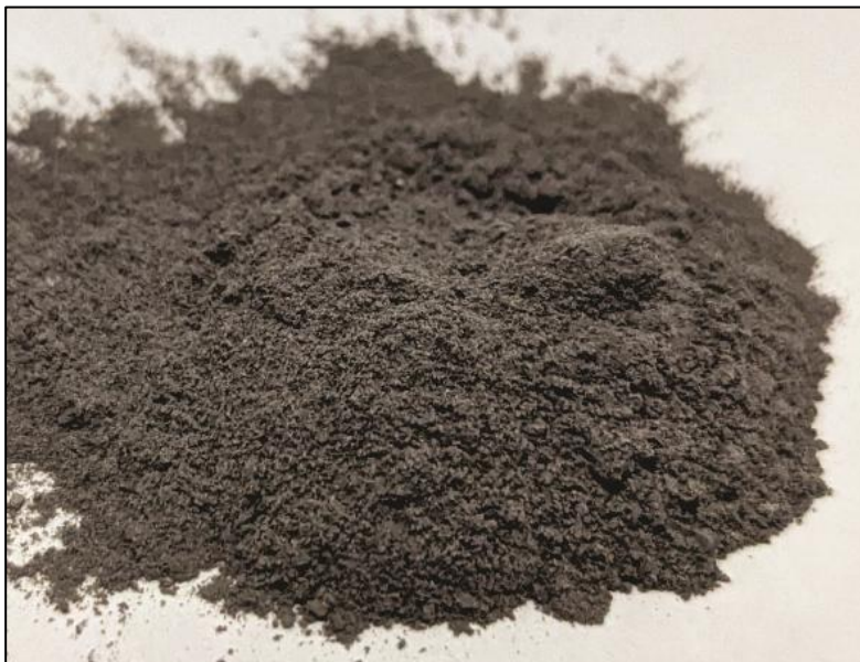
Figure 1: Antimony sulphide (37% Sb) precipitated from leach liquor
