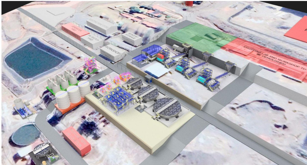
Figure 5: New TGME Plant Layout
