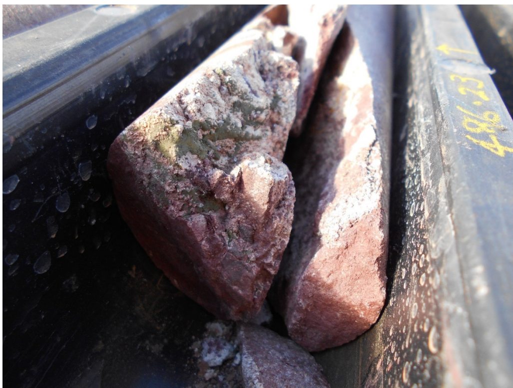
Above and Below: Copper sulphides are irregularly distributed through the breccia, and are most prominent in vugs, on fracture surfaces and associated with quartz veining.
