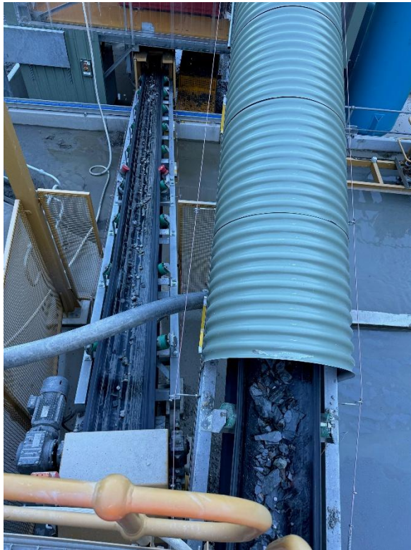
Figure 3. The Ore Sorter performed as expected with the trial hard rock ore
