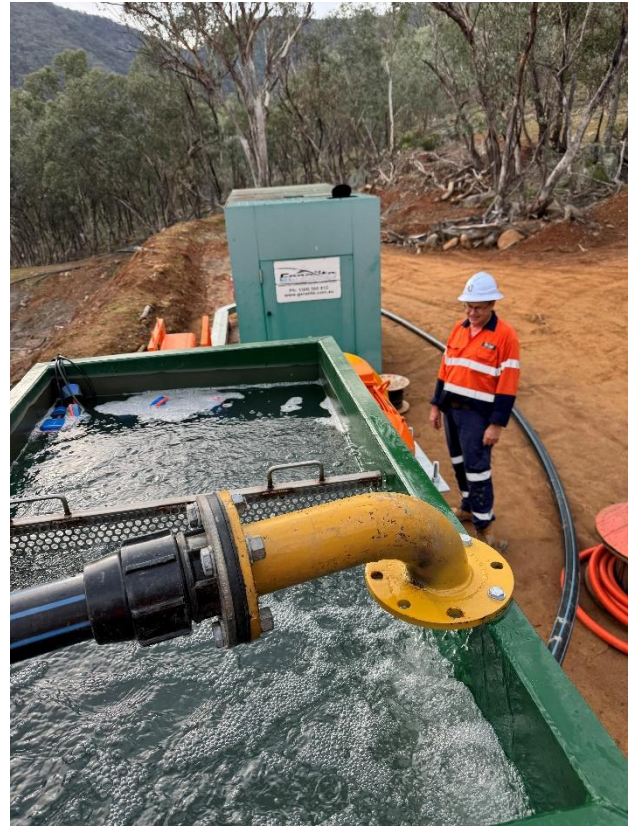
Figure 8 Clear fresh decanted water ready to be pumped back from the sand stack to the Reward Gravity Gold processing plant.
