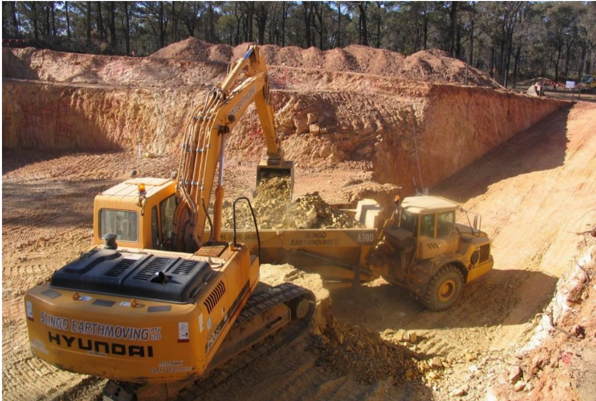
Figure 3 - Excavating bulk sample pit at Harvest Home
