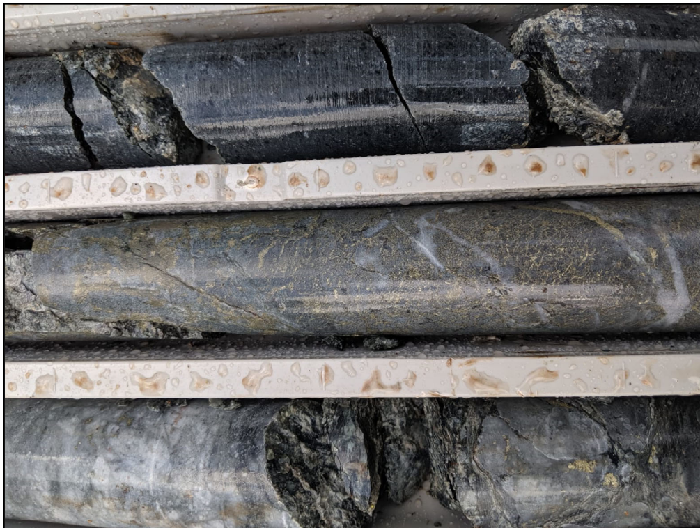
Figure 2 : Hole 1, NQ Core, disseminated and vein chalcopyrite (yellow) within diorite at 17.2m (centre core).
