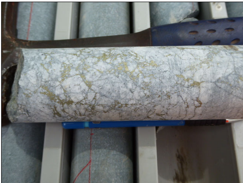
Figure 4 : Hole 1, NQ Core, chalcopyrite and some bornite within matrix of diorite breccia at 26.7m.
