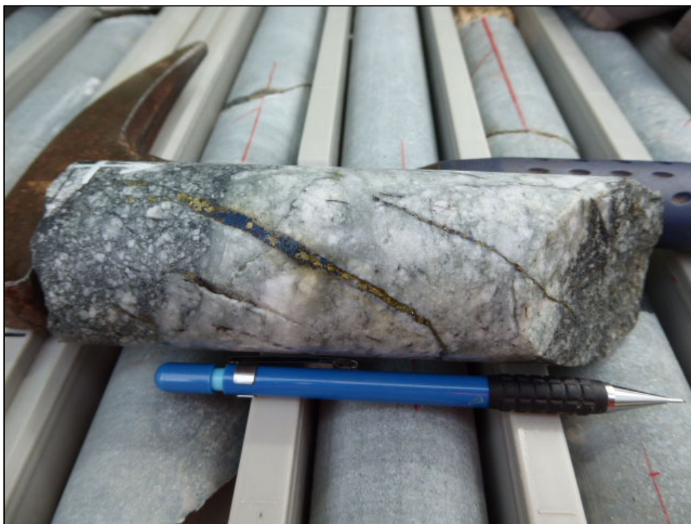
Figure 3 : Hole 1, NQ Core, late veins of bornite (purple to blue) chalcopyrite (yellow) within diorite silicified breccia at 18.7m.
