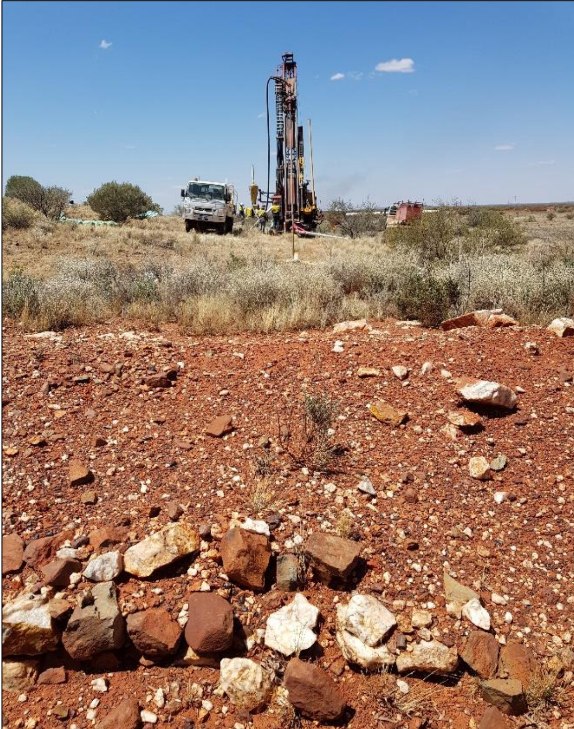
Figure 13: Photo showing RC drilling in operation at Dover Castle South.
