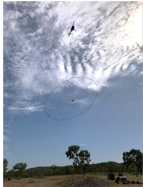
Plate 1: VTEM Survey in progress May 2022
