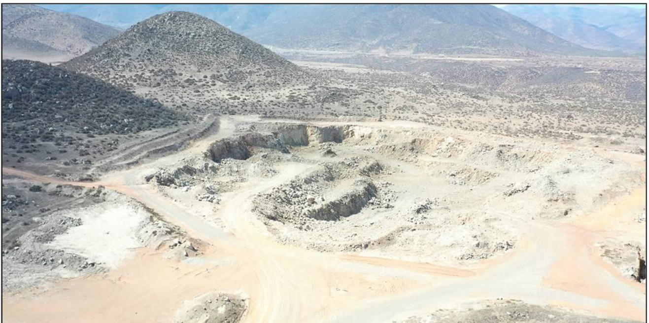
Figure 2 - Drone image of trial mining pit looking NE. Eighteen RC drill holes drilled in and around pit area.
