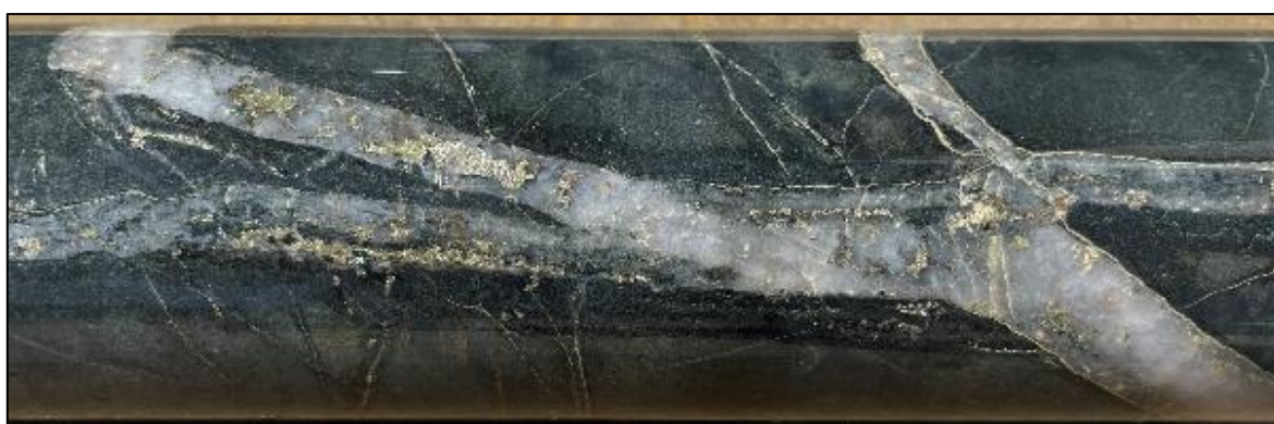
Photo 11. Quartz-chalcopyrite-pyrite veins in basaltic andesite. Magnetite (not seen) also occurs in these veins, STWD007 at 290.65m - 1m at 0.25% Cu within 27m at 0.14% Cu from 268m.
