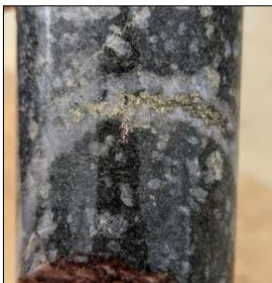
Photo 6. Quartz pyrite chalcopyrite vein - STWD006 at 124.2m.
