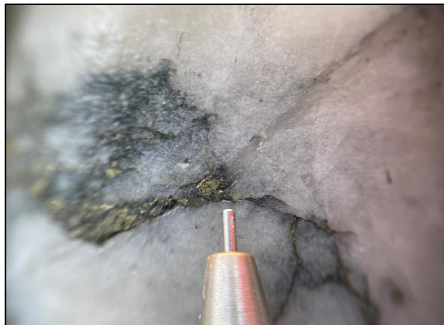
Photo 4. Same vein as above showing silvery-grey aggregate that is probably tetrahedrite, STWD005 at 287m - 0.6m @ 8.72g/t Au, 1.85% Cu, 5.2g/t Ag & 151ppm Mo.
