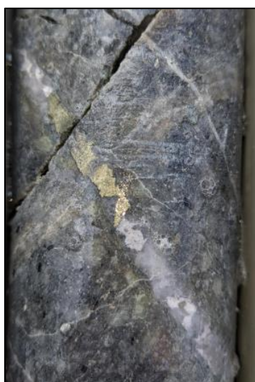
Photo 9. Quartz chalcopyrite vein - STWD006 at 137.6m.
