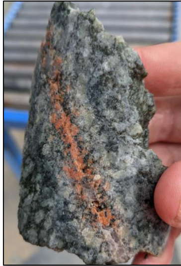
Photo 1. Potassium feldspar selvage, around a quartz vein with very trace chalcopyrite and pyrite - STWD005 at 139.8m.
