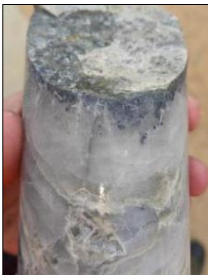
Photo 7. A 50mm wide quartz-molybdenite (silvery-blue sulphide) vein - STWD006 at 130.5m.
