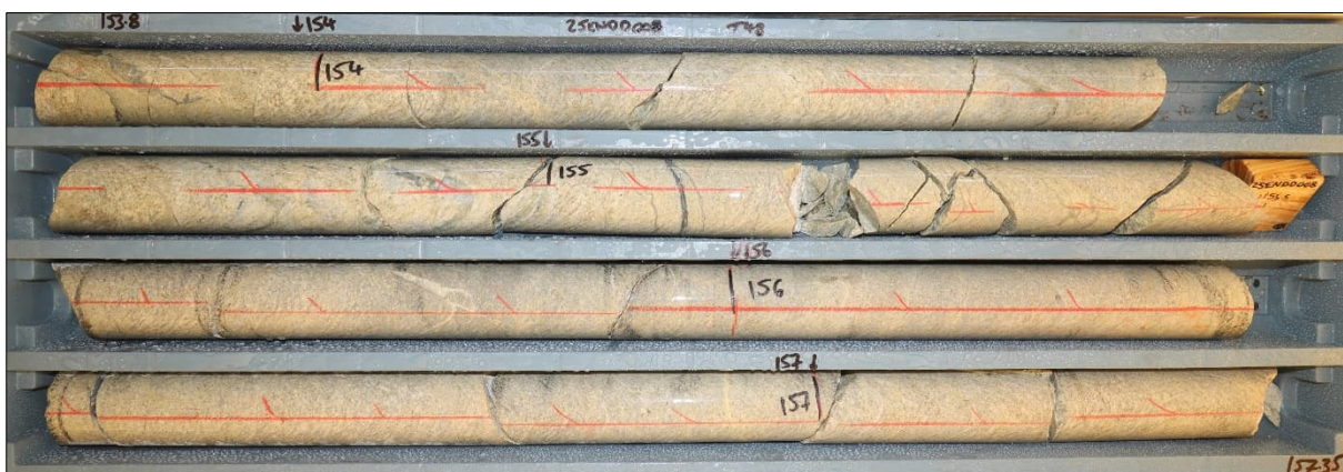
Photo 5 - Hole 25ENDD008 from 153.8-157.35m. Strongly phyllic altered medium grained foliated granite with buff coloured Iron Carbonate-quartz-(Py) veins, some with reasonably high sulphide content.
