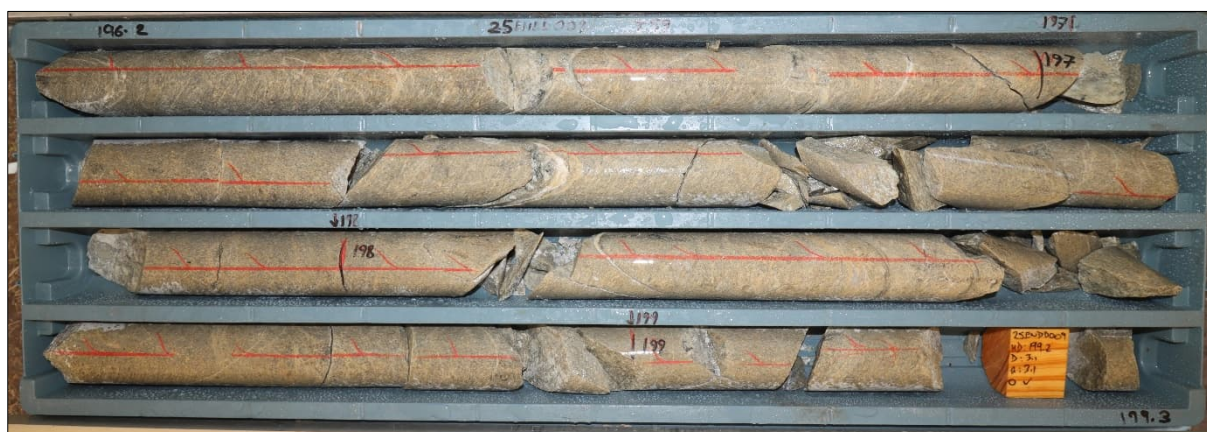
Photo 8 - Hole 25ENDD009 from 196.2-199.3m. Strong selectively pervasive Fe carbonate-quartz-pyrite-sericite-arsenopyrite altered, medium grained, bleached, sheared, granite. Sulphide rich quartz-carbonate vein set with notable arsenopyrite and rare fine dark grey/black sulphide (sulphosalt?).
