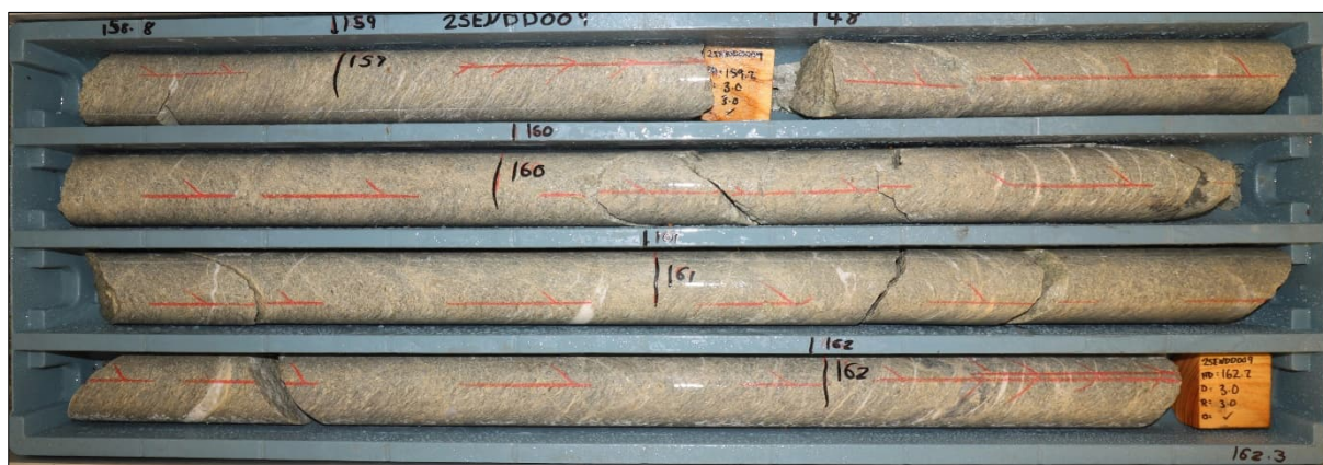
Photo 7 - Hole 25ENDD009 from 158.8-162.3m. Strong selectively pervasive Fe carbonate-sericite-quartz-pyrite altered, medium grained, bleached, sheared, granite. Sulphide rich quartz-carbonate vein set with notable arsenopyrite.
