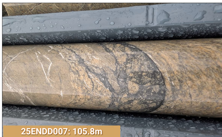
Photo 1. Sample photo of 25ENDD007 at 105.8m with iron carbonate alteration and sulphide breccia-vein array. Diameter of drill core is 61.1mm.
