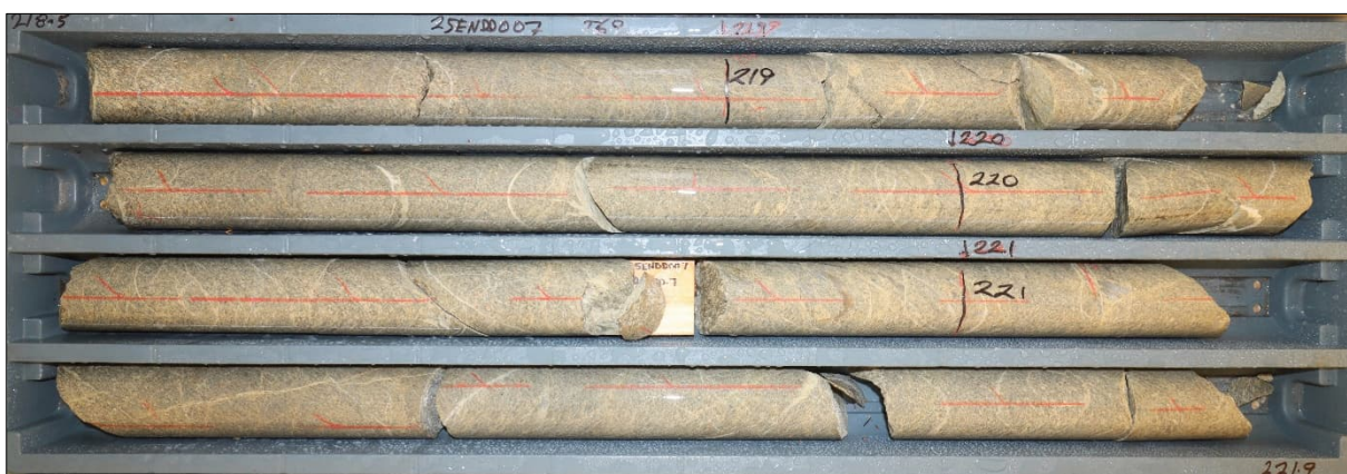
Photo 4 - Hole 25ENDD007 from 218.5-221.9m. Strongly phyllic altered granite with mostly brecciated quartz-carbonate veins with a strong enrichment in Py ± As sulphides.
