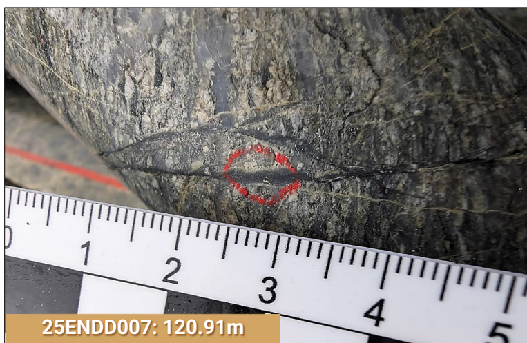
Photo 2. Sample photo of 25ENDD007 at 120.91m with visible gold in late stage, extensional, flat-dipping, drusy quartz vein cross-cutting the shear fabric. Numerical units on scale bar are centimetres. Refer cautionary note regarding visible gold.
