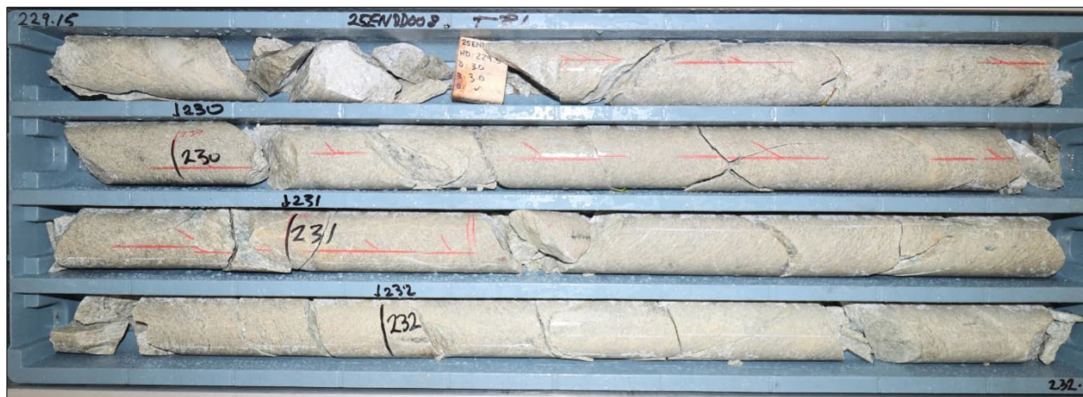
Photo 6 - Hole 25ENDD008 from 229.15-232.6m. Pervasive phyllic alteration in granite with quartz-carbonate veining and disseminated pyrite.
