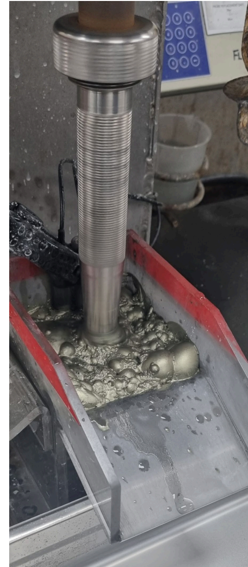
Caravel ore laboratory scale flotation testwork
