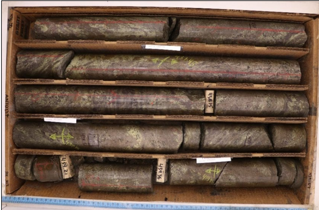
Figure 2 – ANT137 Massive Sulphide Mineralisation (436.55m to 439.67m)
