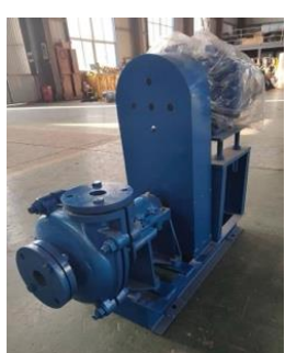
FILTER PRESS PUMP
