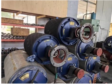
DRUM PULLEYS
