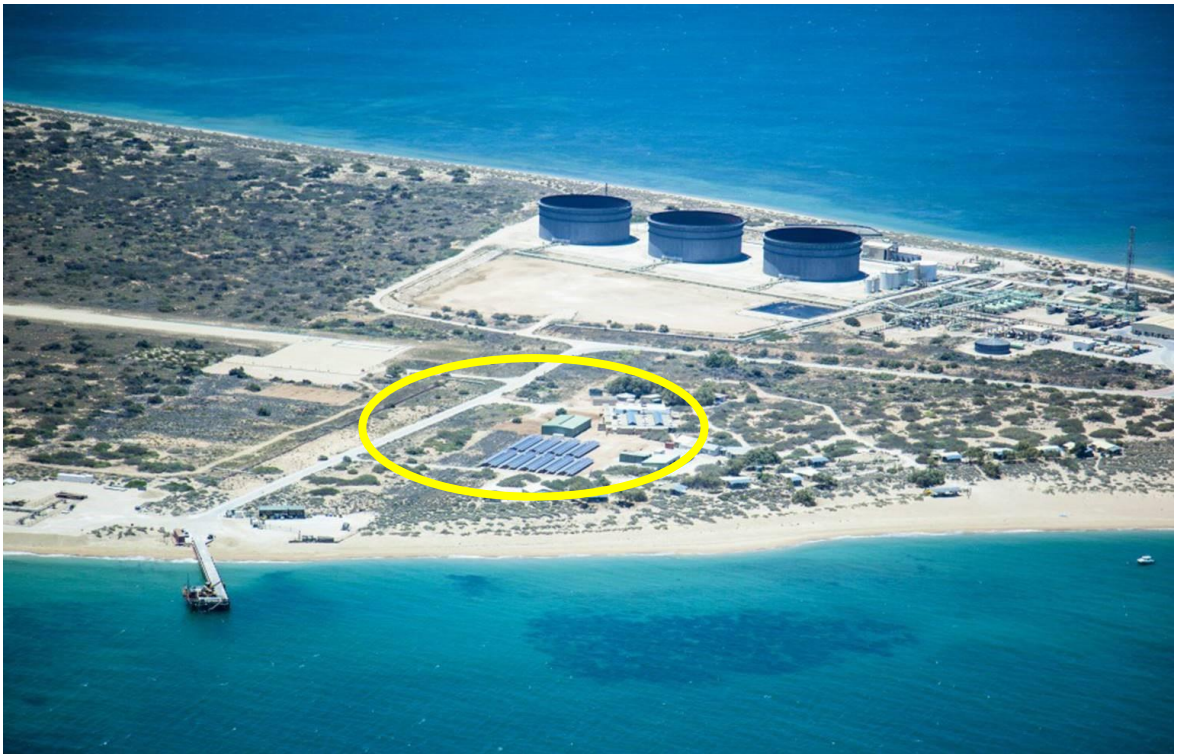
EMC's Mackerel Island project incorporating 320kW of sola, 640kWh of lithium ion battery storage and four back-up generators
