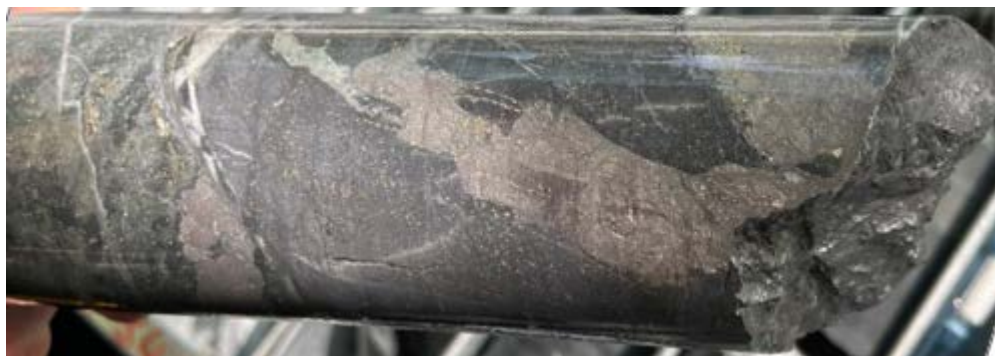
High grade sulphide (arsenopyrite, pyrrhotite and pyrite) mineralisation in RCDD22OKV444 at 323.5m from intersection - 6m @ 14.10g/t from 323m at Okvau Gold Project
