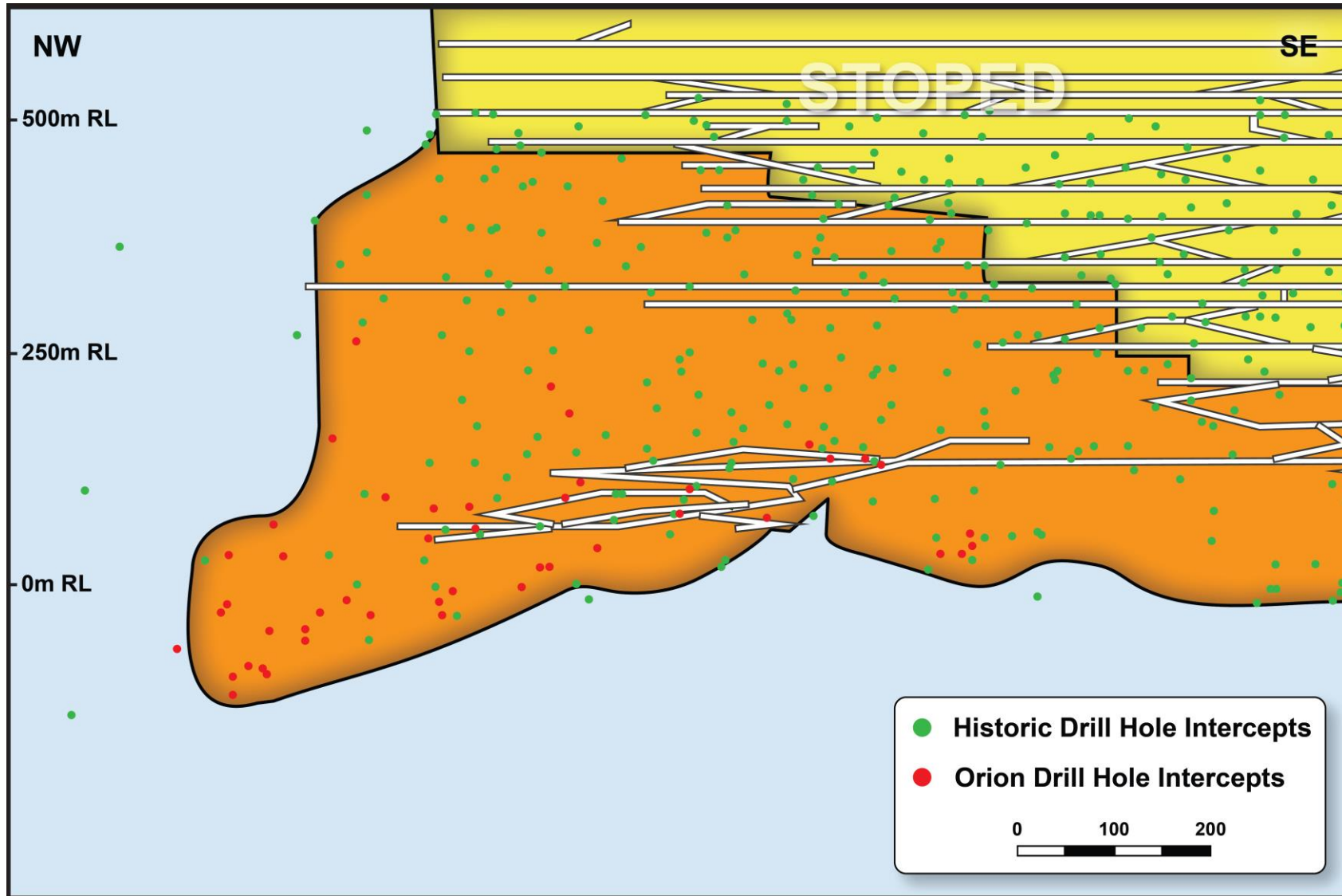
Figure 3A: Longitudinal projection of the North-West Resource area of the Prieska Project, showing the intersection points of the drill holes used in this Mineral Resource release.
