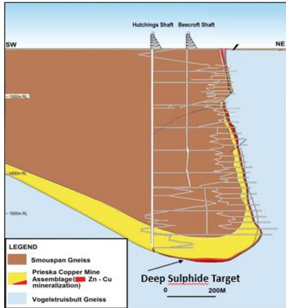
Figure 2A: Simplified geological section through Prieska Project showing structure and locality of the Deep Sulphide Target below the old workings.
