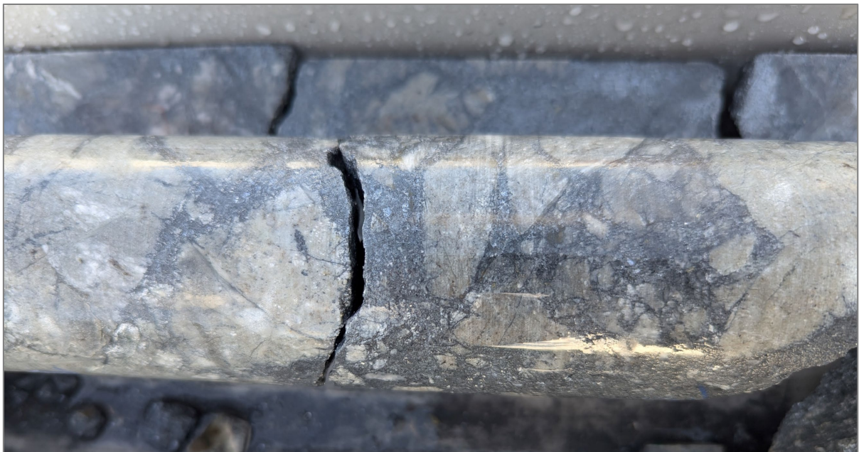
Figure 19: Core photo of the high-grade Sb interval in RDRC067 highlighting brecciated ultramafic at 239.4m. Refer ASX Release 26 August for full context)
