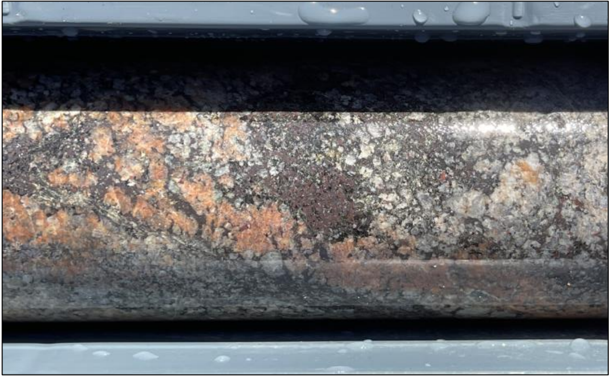
Figure 3. Photo showing an example of granite found in drill core from Central DDH003.
