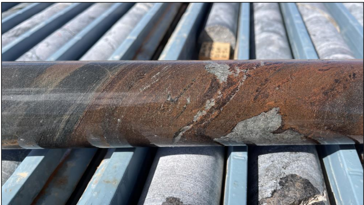
Figure 4. Photo of HQ diamond drill core CENTRAL_DD003 showing hematite staining of country rocks.
