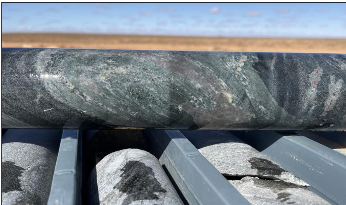
Figure 1. Initial first-pass observation of stage 2 hydrothermal alteration of host rocks. Initial observations indicate epidote-chlorite-sericite +/- actinolite and biotite alteration. Diamond HQ drill core Central_DD003.
