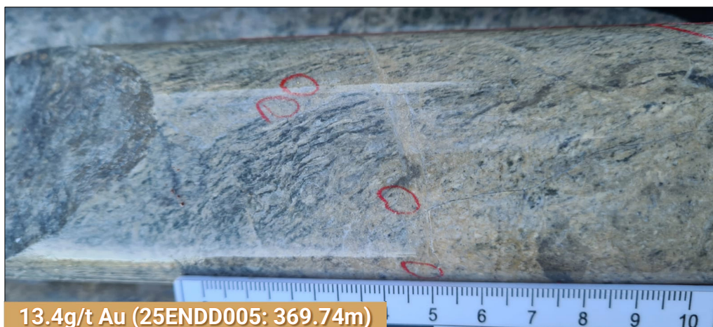
Photo 3. Sample photo of 25ENDD004 from 369.6m – 370m @ 13.4g/t Au with visible gold circled in red associated with Fe-Carbonate quartz-pyrite-arsenian pyrite + adularia veins within granite host rock. Numerical units on scale bar are centimetres
