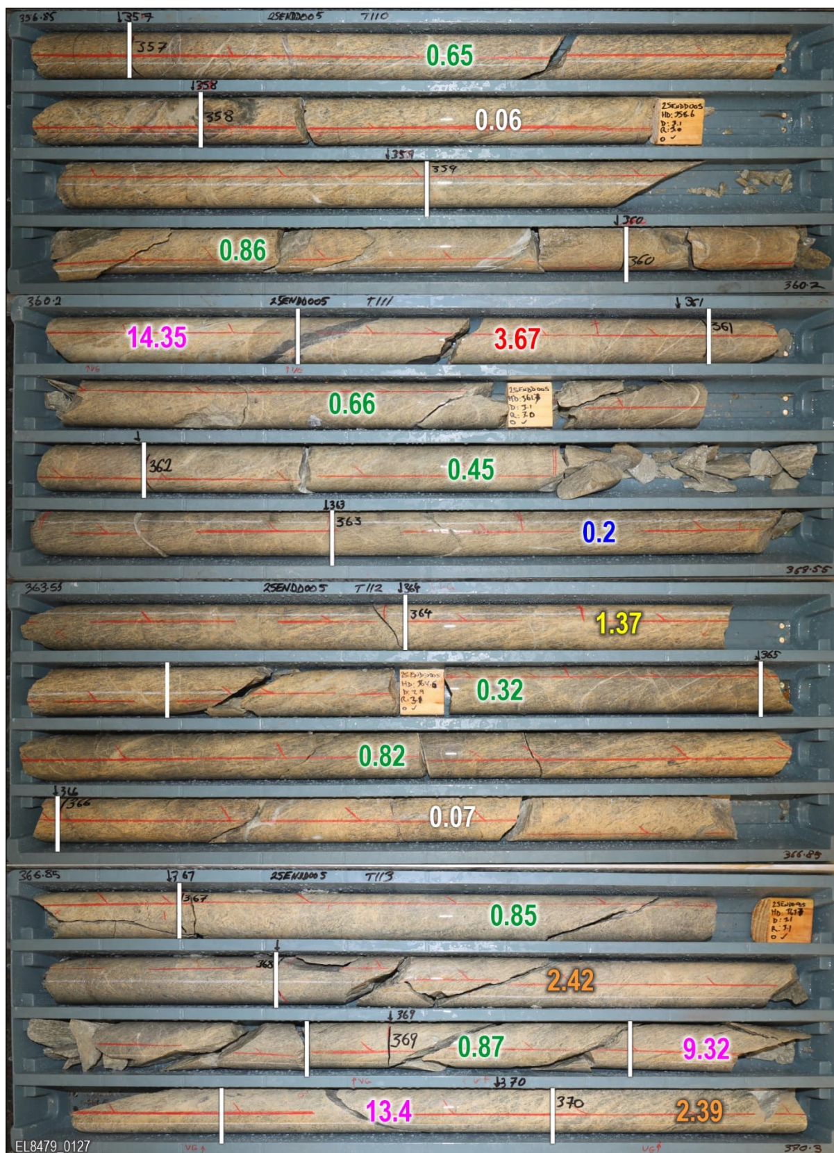
Photo 5 (continued from previous page). Core tray photos of 25ENDD005 interval 21m @ 1.65g/t Au from 356m incl. 10.4m @ 2.36 g/t Au from 360m. Distinctive paler coloured zones (silica-sericite altered) typically host better grades (although not exclusively) and are interpreted to have overprinted the darker coloured zones (propylitic/chlorite altered). The numbers superimposed on the core are the reported gold assay grades over each respective sample interval.
