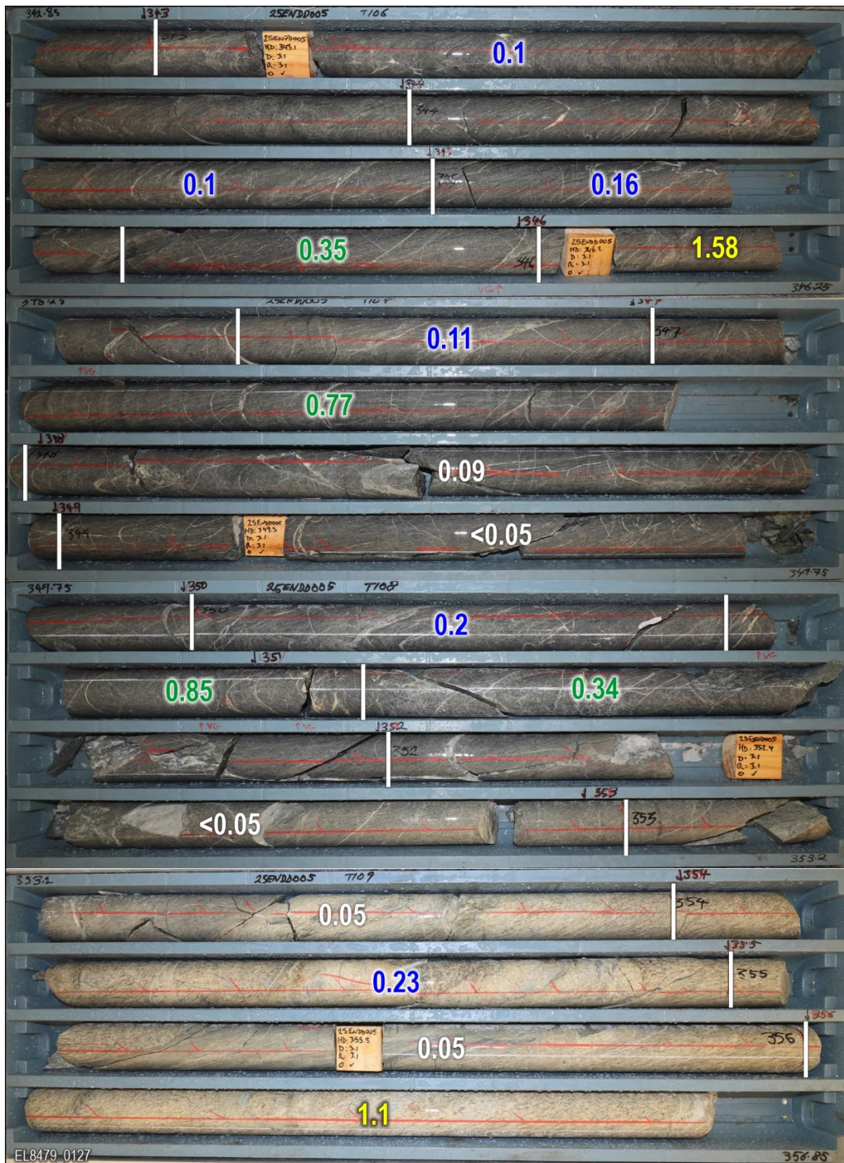
Photo 4. Core tray photos of 25ENDD005 interval 21m @ 1.65g/t Au from 356m incl. 10.4m @ 2.36 g/t Au from 360m. Distinctive paler coloured zones (silica-sericite altered) typically host better grades (although not exclusively) and are interpreted to have overprinted the darker coloured zones (propylitic/chlorite altered). The numbers superimposed on the core are the reported gold assay grades over each respective sample interval.
