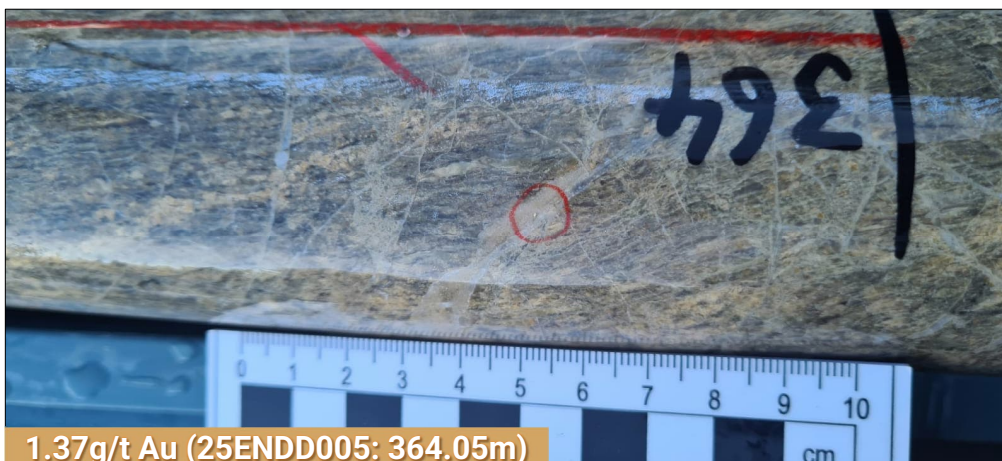
Photo 2. Sample photo of 25ENDD005 from 364m – 364.5m @ 1.37g/t Au with visible gold circled in red associated with quartz-iron carbonate-pyrite-arsenian pyrite +adularia veins in granite host rock.
