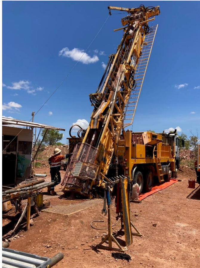
Figure 2: DDH1 – Geotechnical Drilling
