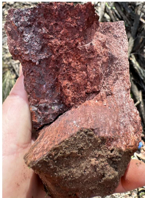
Figure 2 – Silver mineralisation within ferruginous sandstone yielding 73.4 g/t Ag , & >1% Ba from sample 3000996
