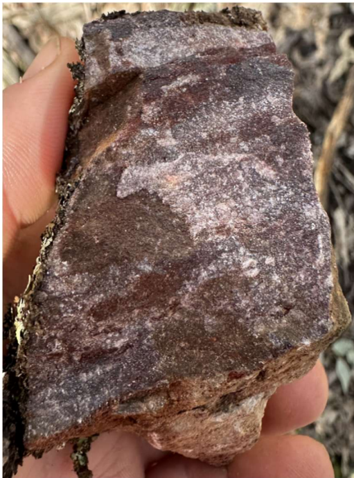
Figure 1 – Silver mineralisation within ferruginous barite outcrop yielding 117 g/t Ag , & 0.26% Ba from sample 3001009
