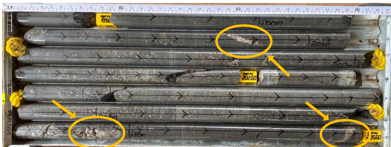
Figure 2 Zone of blebby and heavily disseminated sulphides with occasional semi-massive veinlets intersected from 200.7m depth in drill hole DDLUHC002
