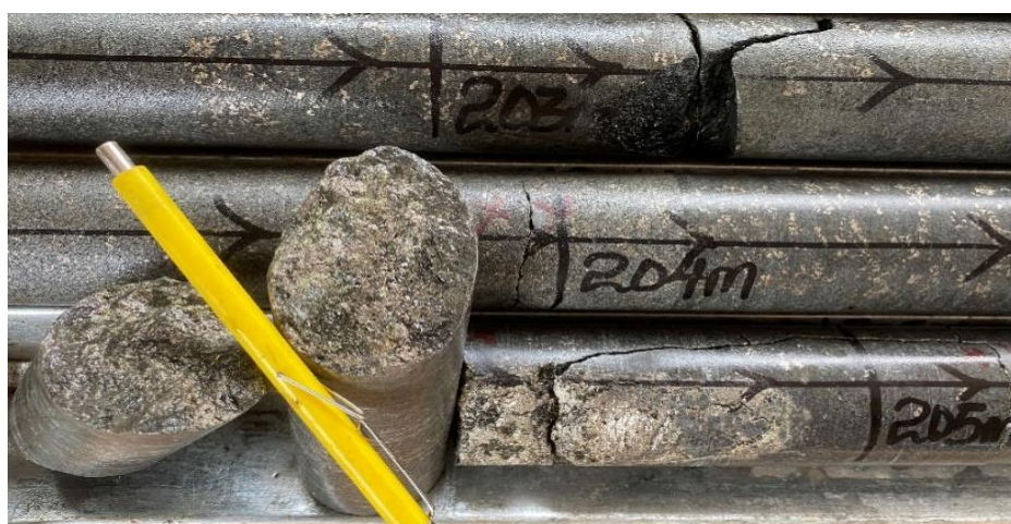
Figure 1 Section of the 4.9m intersection of heavily disseminated and semi-massive sulphide hosted in gabbro-norite
