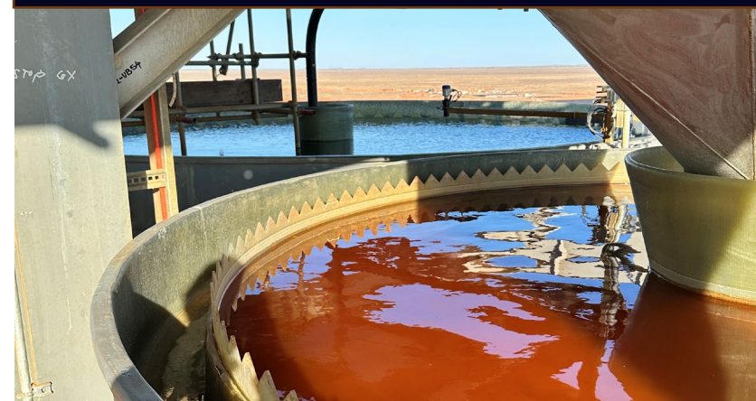
IX Adsorption and Elution Columns – A Train
