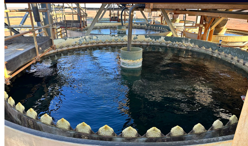
Top of IX Adsorption Column C
