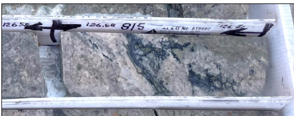
Figure 1. Cut portion of diamond core from YQ-25-001 at ~126.6 metres down hole. The interval forms part of the lower Pertenencia Vein intersection and comprises a breccia infilled by silver-bearing sulphide mineralisation (black), grading 0.13m at 2,250g/t Ag & 17.2g/t Au (3,569g/t AuEq) 1 .
