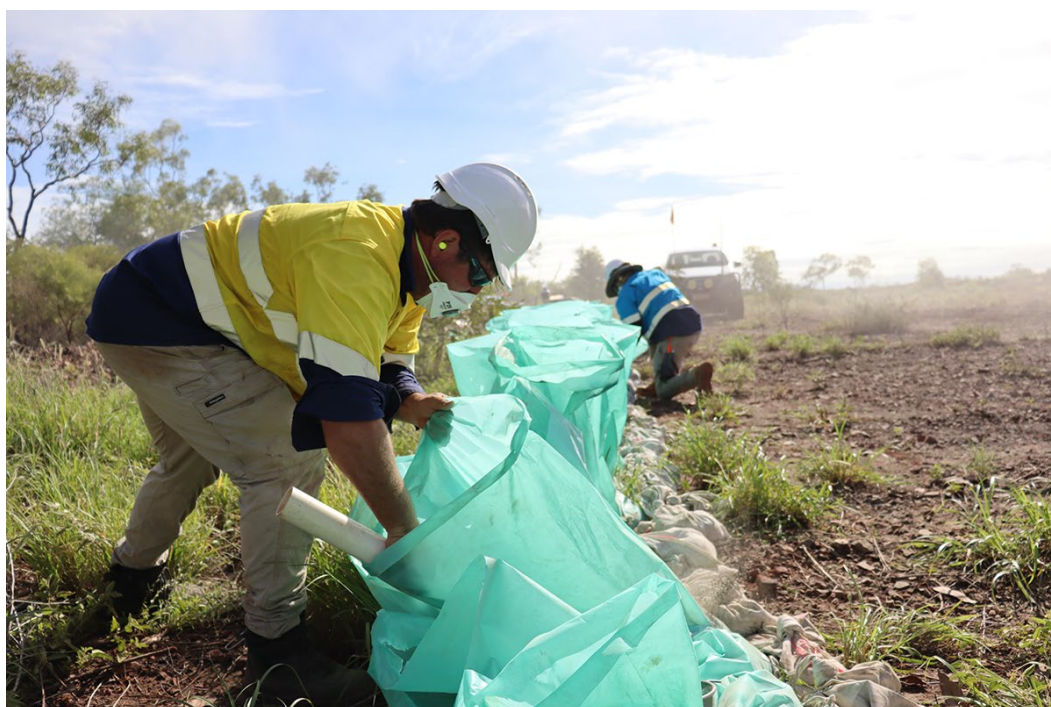
Photo 2. Sparging sample with PVC for the geological chip logging.
