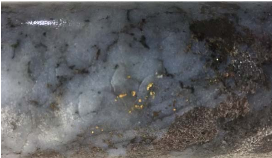
Visible gold in core at Challenger West
