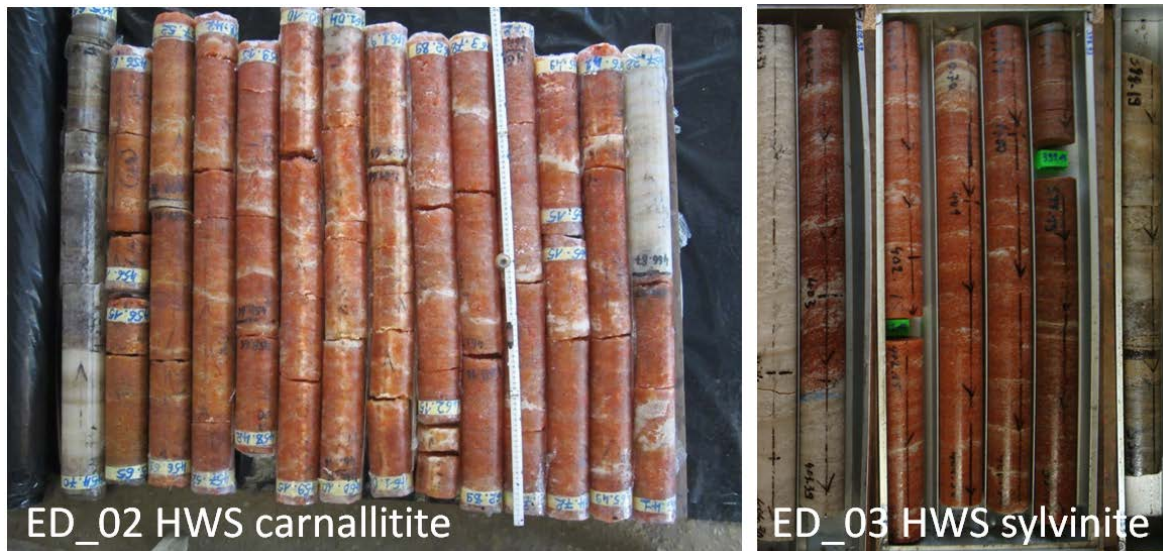
Figure 2. Left: Carnallite Hangingwall Seam in drillhole ED_02. This interval grades 24.65 % KCl (15.56 % K 2 O) over 11.2 metres and is comprised of 90% carnallite. Right: Sylvinitic Hangingwall Seam in ED_03 grading 59.48 % KCl (37.56 % K 2 O) over 4.2 metres. Note excellent core recovery and horizontal layering throughout.
