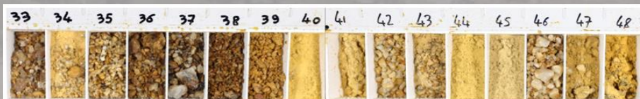
Photo 1: NMWBAC24-721: 4m @ 6.85 g/t Au (from 44m) within 16m @ 2.74 g/t Au (from 32m)
