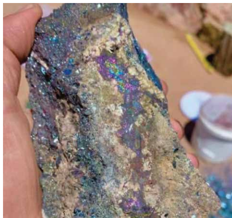
Figure 14. IOCG mineralisation in hematite-breccias, outcropping at the Flinders Project.
