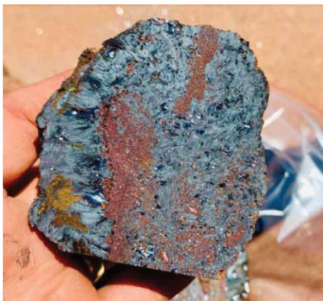
Figure 14. IOCG mineralisation in hematite-breccias, outcropping at the Flinders Project.
