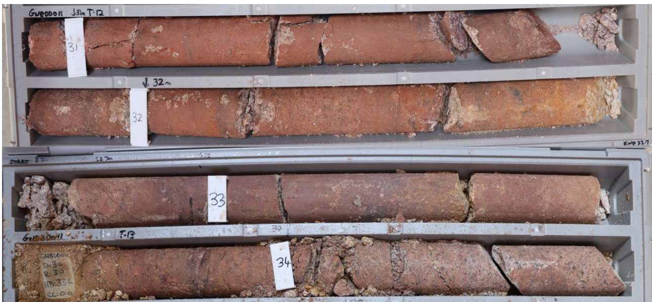
Figure 3: Clay weathered saprock in diamond drill core GNBDD011 3m @ 3481ppm TREO i from 31m.
