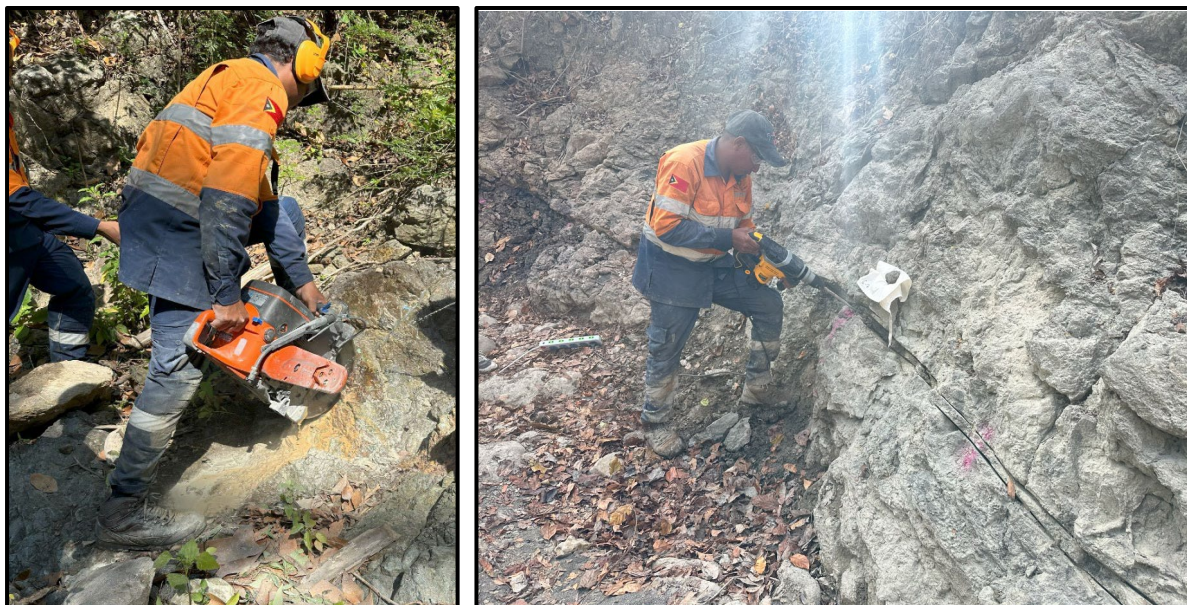
Figure 4 A-B: Systematic channel sampling of mineralised outcrops using a diamond saw and electric impact chisel. Assays of channel sampling undertaken at this and other locations are currently pending.
