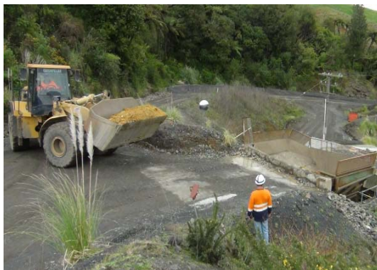
Talisman ore being fed into Crusher
