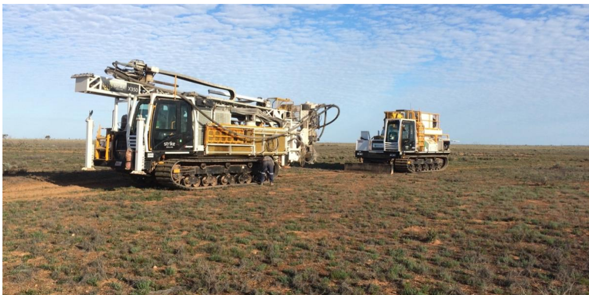
Figure 3: Strike Drilling Morooka based Aircore drilling rig and support vehicle.
