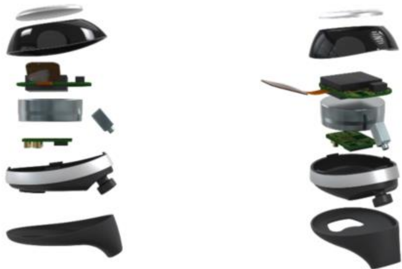
Figure 1 - Nuheara preliminary ear-bud hardware design
