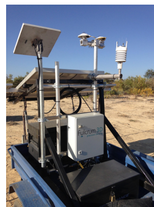
Solar monitoring station at Kidston
