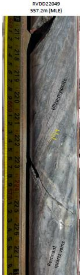
A strongly developed ultra-mylonitic fabric around sheared and boudinaged quartz veins in the Main Lode East structure. Sulphides remobilised around quartz veins and into "pinched" boudin necks. NB relatively long boudin neck, an indication of the degree of stretching during deformation.
