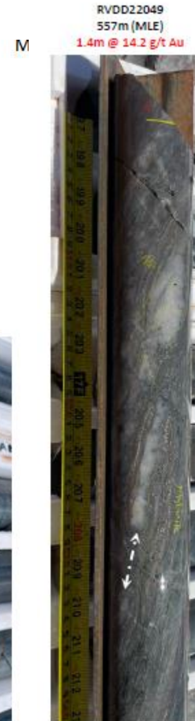
A strongly developed ultra-mylonitic fabric around sheared and boudinaged quartz veins in the Main Lode East structure. Sulphides remobilised around quartz veins and into "pinched" boudin necks. NB relatively long boudin neck, an indication of the degree of stretching during deformation.
