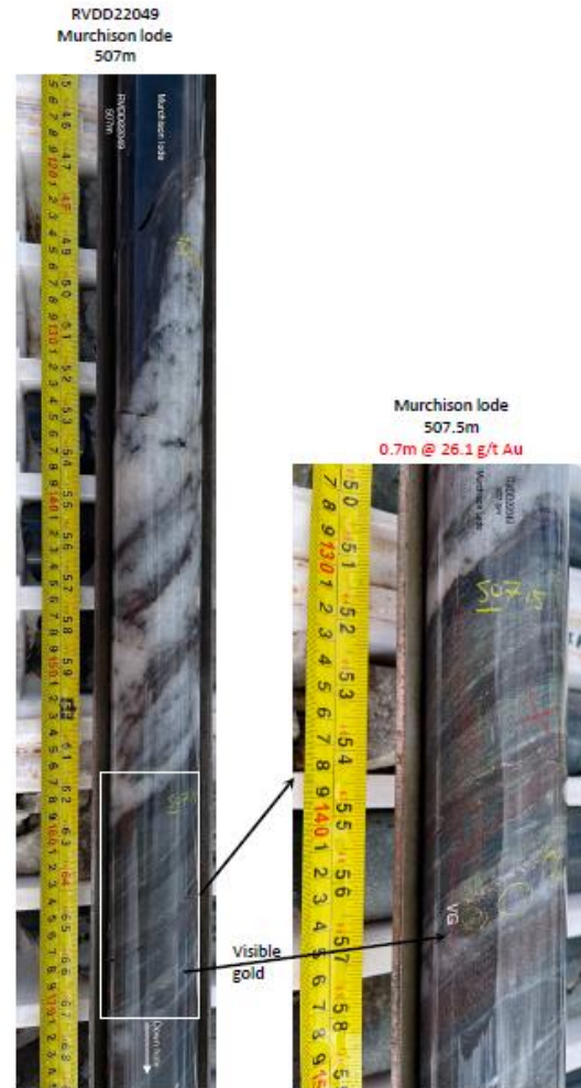
A well-developed Murchison lode with visible gold concentrated in a mafic band adjacent to a boudinaged quartz vein. Strong mylonitic texture developed in the FW of the zone of sheared quartz.
