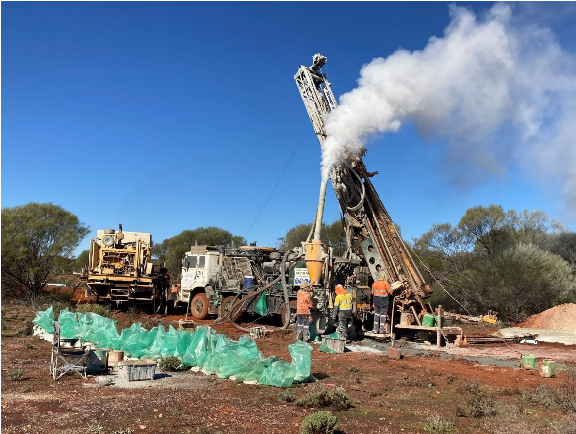
Plate 2: Reverse Circulation drill rig on site at Yidby Gold main zone.
