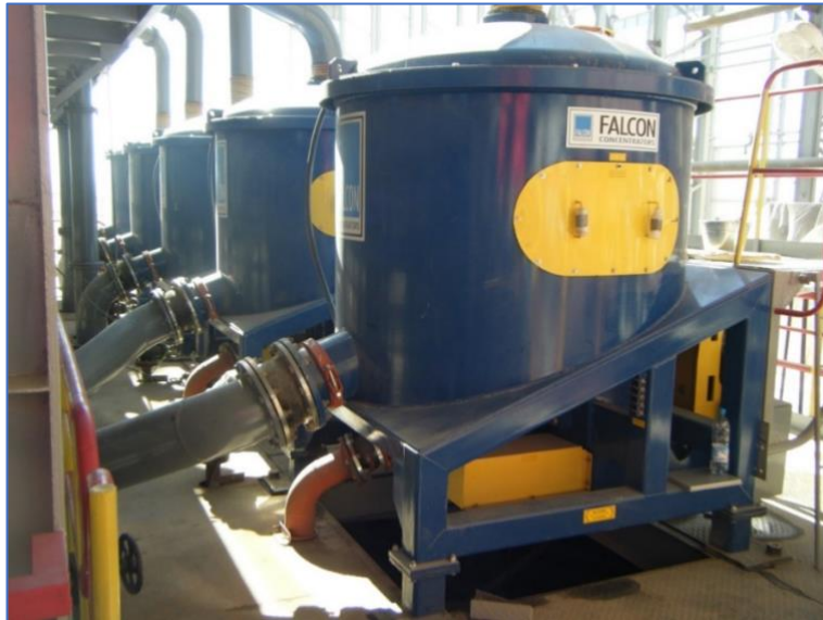
Figure 82. Falcon SB5200 centrifugal gold concentrator modules
