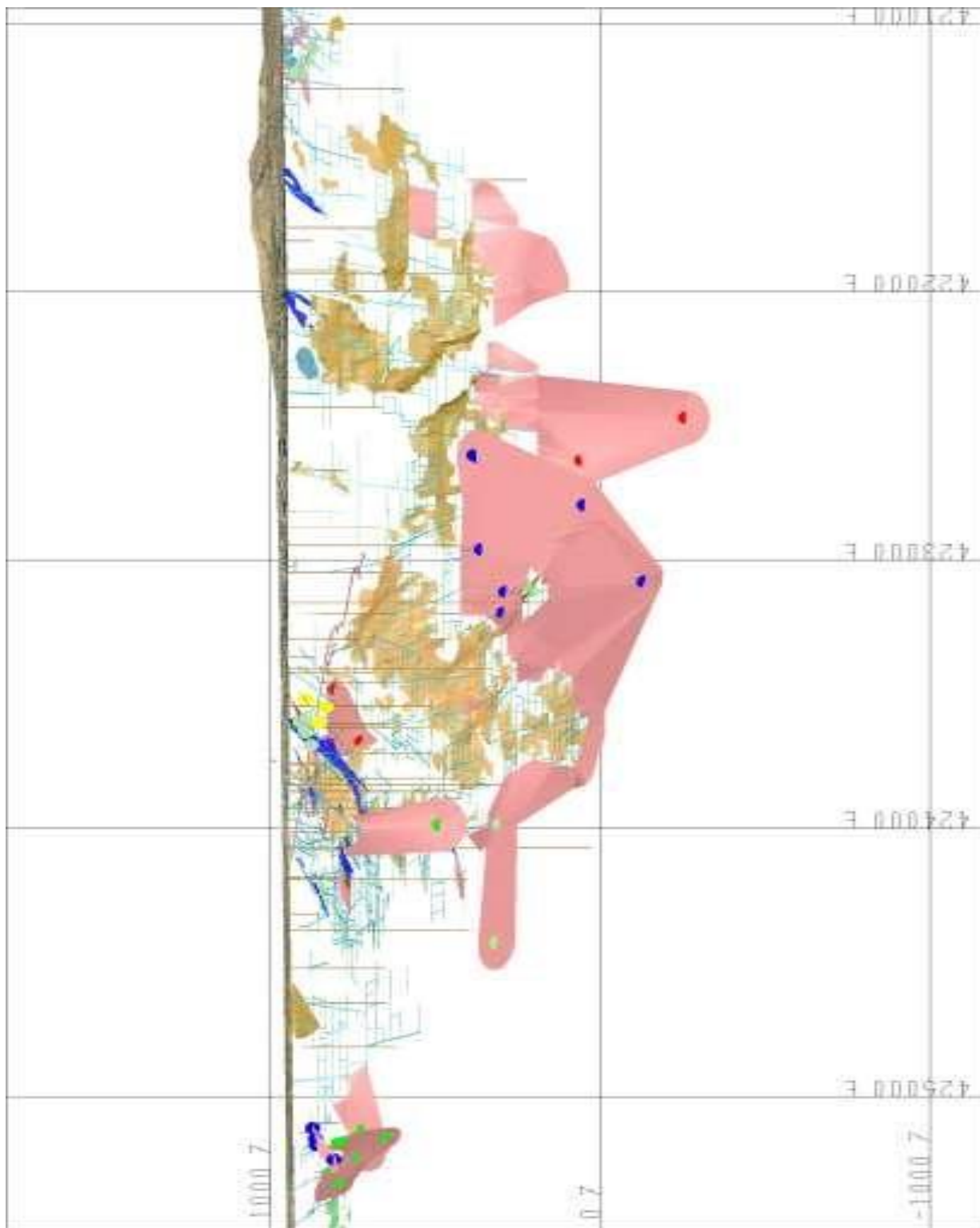
Figure 66. Long section looking south, showing the drill pierce points through the Central Area Indicated Mineral Resource structures.
