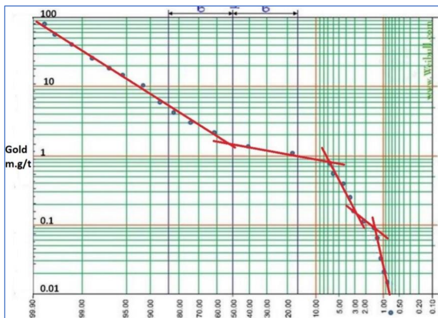
Figure 40. Log Probability plot of 1,559 drill intersections. It shows a background population below 0.1 m.g/t Au, one mineralising population from 0.3 to 1 m.g/t and a high grade mineralising population above 1 m.g/t Au.
