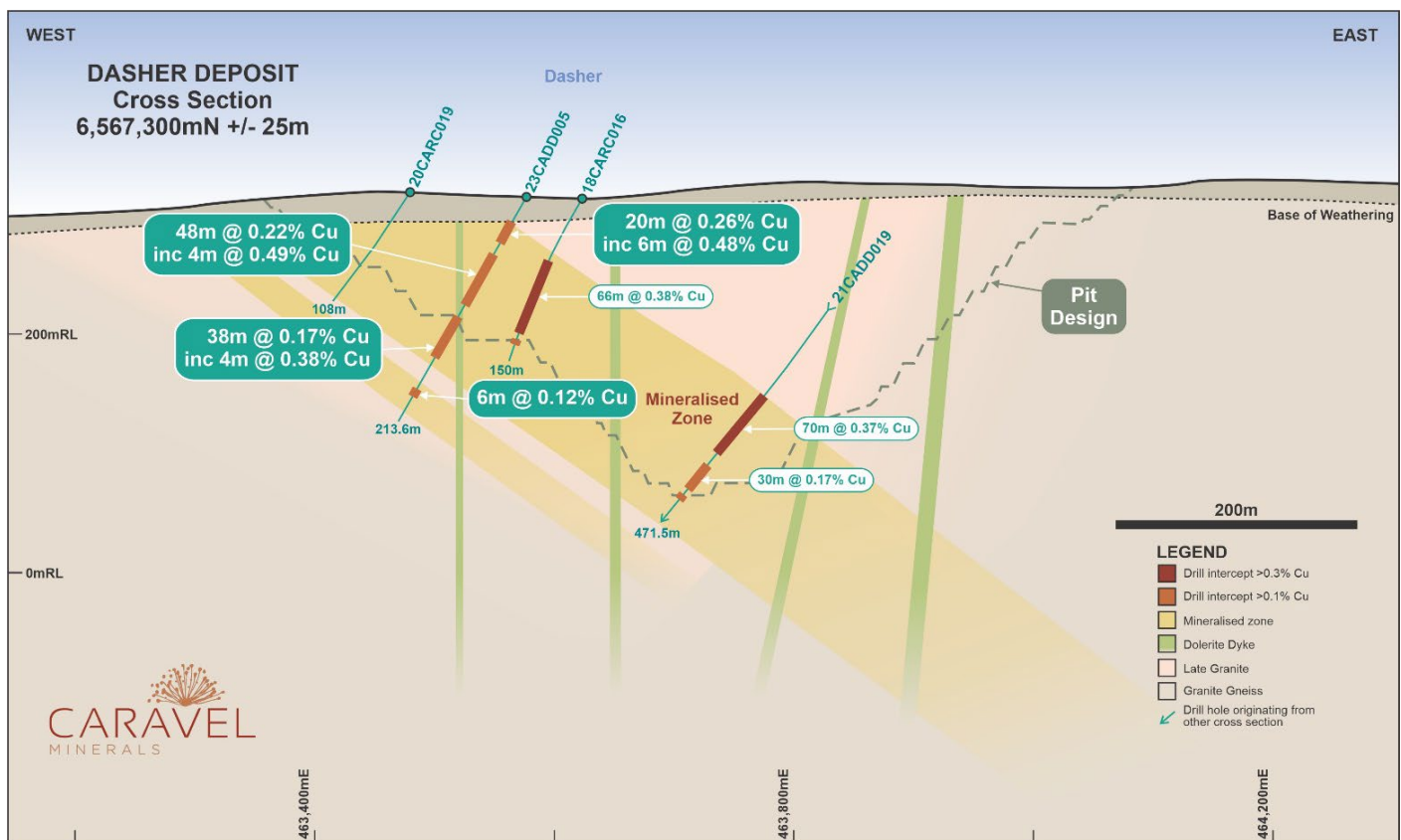
Figure 6: Dasher Deposit cross section 6,567,300N looking north, illustrating recently completed drill holes 23CAD005
