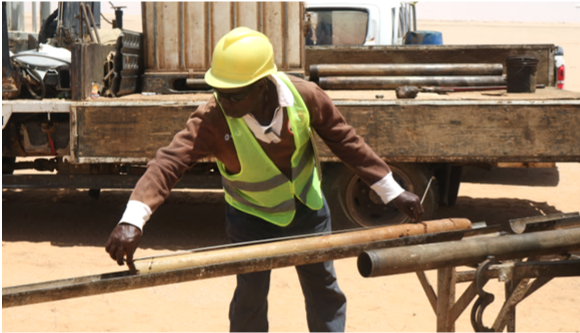
Figure 10 – Drilling contractors at Tiris checking core recovery
